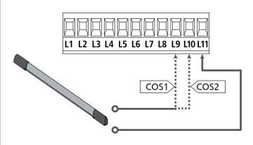
In order to meet the requirements of the EN12978 rules, it is necessary to install safety edges controlled by a control unit continuously checking the proper working. If using control units suited to the test by power outage, connect the power supply cables of the control unit between terminals Z3 and Z2 of the control unit.
