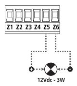
CAUTION: Pay attention to the polarity of the connected device if necessary
