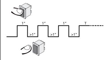
The fourth START command activates the gate in MAN PRESENT mode. To move the gate keep the START command pressed for the duration of the operation (time T).
