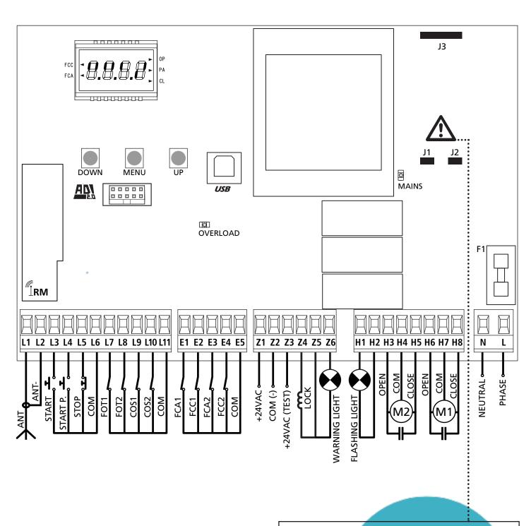
ATTENTION: jumpers J1 and J2 must be removed only to allow connection of the LOW ENERGY optional module. Insert the module only after having disconnected the power supply unit.
